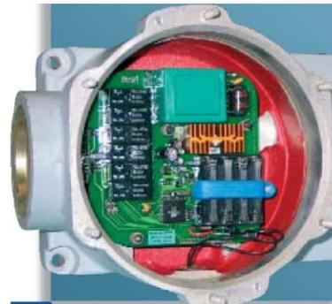
The LSEM is designed to equip types А, Б, В, Г, Д multi-turn electric actuators, serially produced by the TULAELECTRO-PRIVOD, instead of the traditionally used mechanic limit switches module (LSM) and also for part-turn electric actuator 2МПКЭ-4000-С-70.
